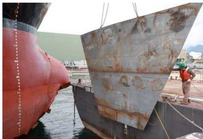
While entering the harbor in the Pacific Northwest a grounding occurred causing significant damage to the forward section of a container ship. After a full underwater inspection was performed by the **Subsea Solutions Alliance** member company from Vancouver, Canada a class approved temporary repair was employed to put the vessel back into service. This temporary repair
